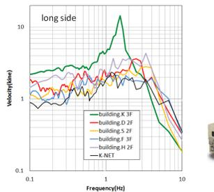
Fig.9 Velocity response spectrum calculated with waveforms recorded by "i-jishin" terminals
